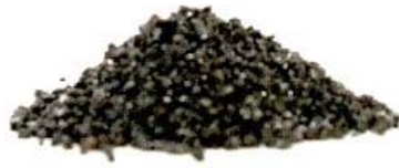
Molten slag made from municipal waste and sewer sludge
