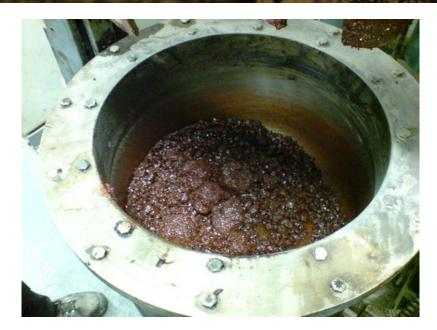
Small particles tend to move downward to the bottom during mixing process
