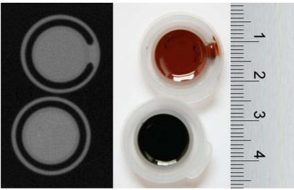
Images taken by X-Ray scanner and normal digital camera of Shell Mexphalte C dyed by 10 % iron oxide and RAP binder
