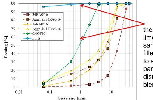
the use of a limestone-crushed sand and mineral filler were required to adjust the particle size distribution of the blend.
