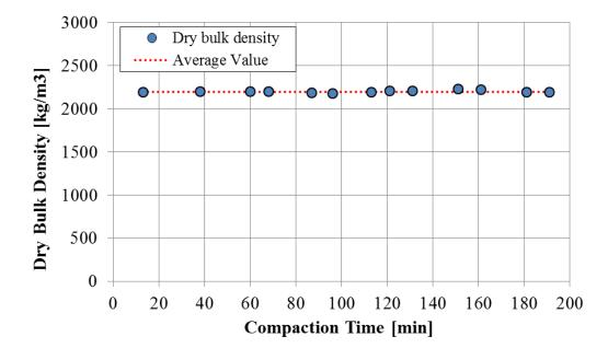
The average dry bulk density was 2200 kg/m<sup>3</sup> and the coefficient of variance was less than 1 %.
