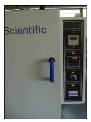
40°C curing temperature ITS specimens – dry to constant mass Triaxial specimens – equilibrium m/c Soaking: 24 hours submerged
