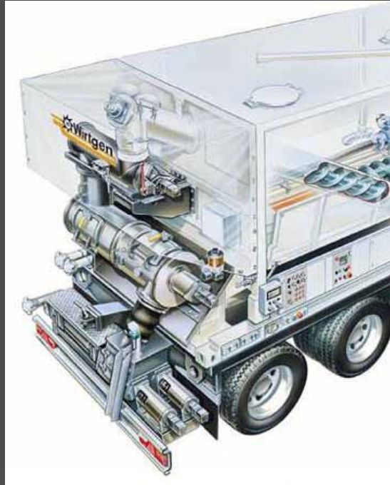
Slurry mixer Cement + Water + Emulsion
