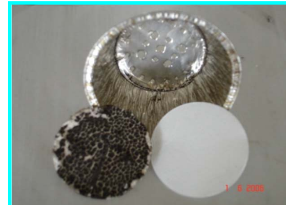
Asphalten contents (ASTM D 3279-97)
