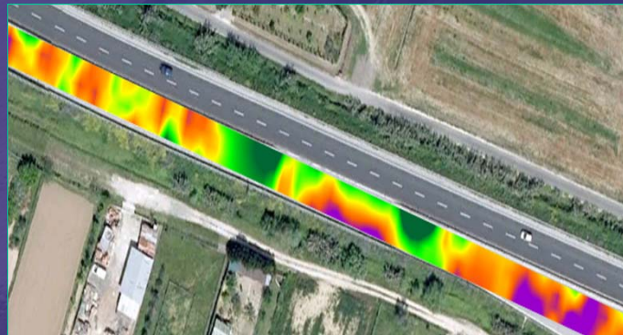
Two-dimensional continuous mapping of the surface tested with LWD can be performed
